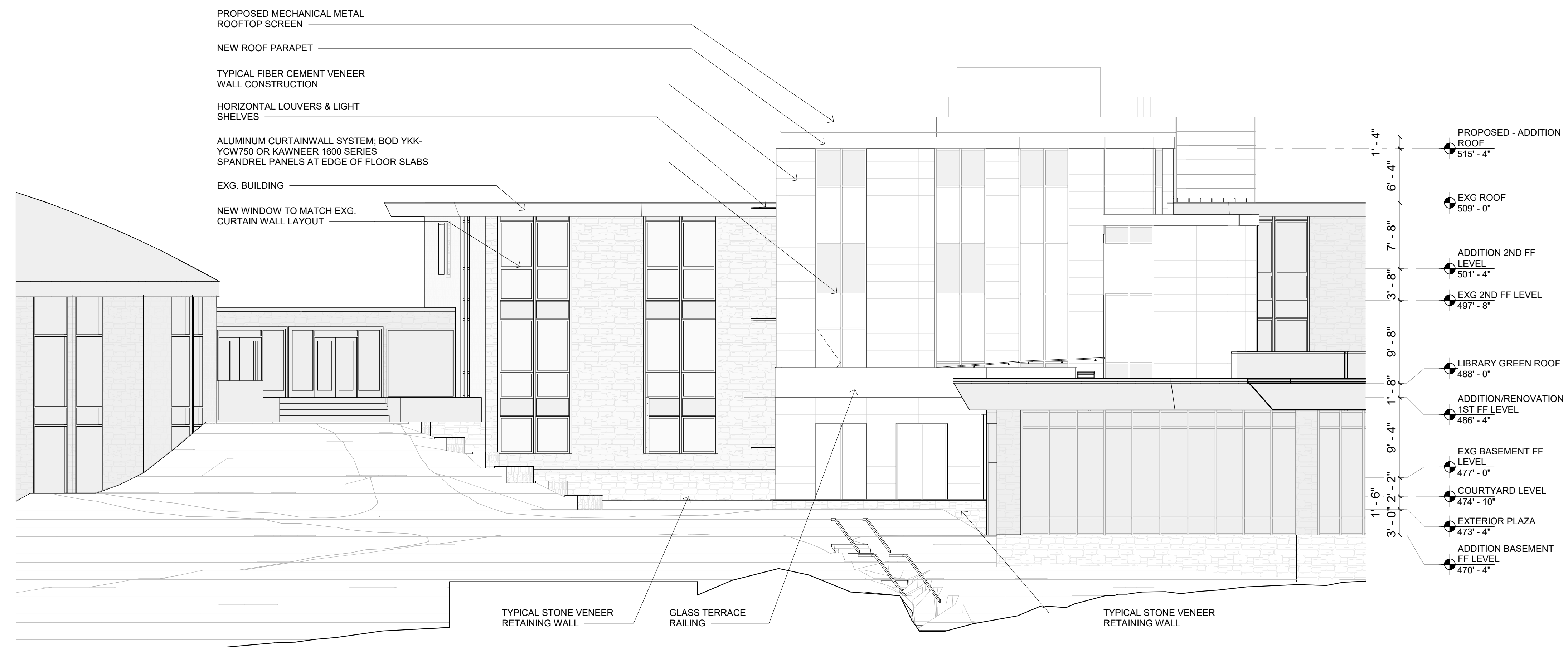
2 EXTERIOR - EAST ELEVATION A3.1 1/8" = 1'-0"
